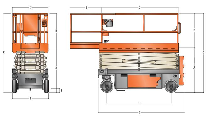
A. Platform Height-Lowered 1.10 m B. Platform Railing Height 1.13 m C. Overall Height (Rails Up) 2.23 m (Rails lowered) 1.80 m
